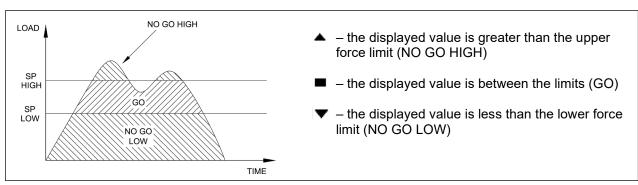
When set points are enabled, the following indicators are shown to the left of the primary reading:
