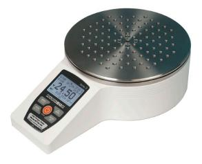
Thank you for purchasing a Mark-10 Series TT05 digital torque tester, designed to measure bottle cap application and removal torque.
